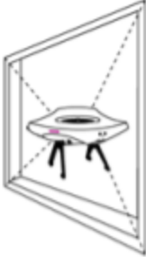
2. Drone enters window through an equidistant center point, using vision and ultrasonic sensors, as well as LiDARs, to keep its distance from the frame.
